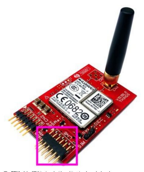
The PIN1 of the CN6 is signed with a white triangle on the board.
