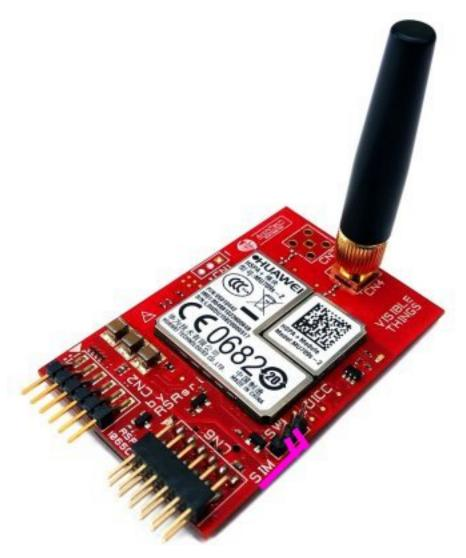
4. Connect board with PMOD interface TYPE 4 to CN6 connector
