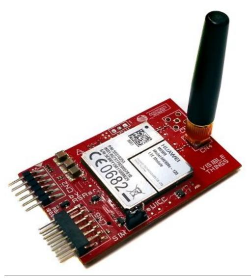
ME909s-120 is the first LTE cat4 module based on Hi-Silicon chipset. Which is high-quality designed LTE module in small size and Huawei standard LGA form factor, especially for industrial-grade M2M applications such as vehicle telematics, tracking, mobile payment, industrial router, safety monitor and industrial PDAs.
