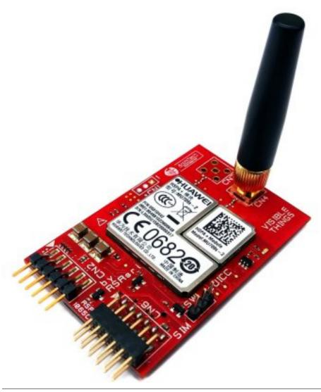
**MU709S2** family is high-quality designed HSPA+ module in small size and Huawei standard LGA form factor which specially for industrial-grade M2M applications such as vehicle telematics, tracking, mobile payment, industrial router, safety monitor and industrial PDAs.
